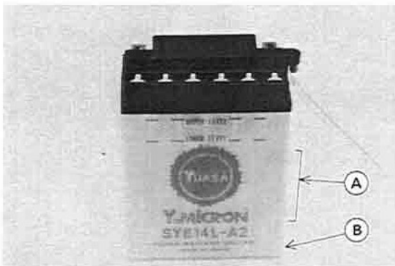
A. Sulfation here B. Sediment here
